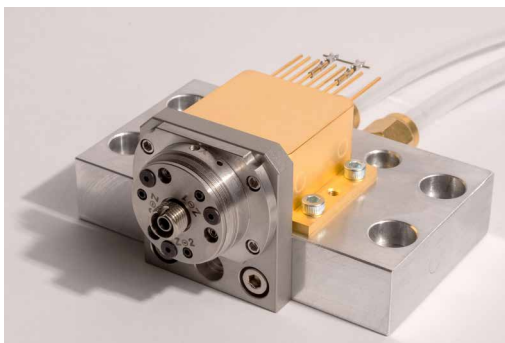
Pigtailed HHL to be delivered with 1-m length of single-mode mid-IR optical fiber. The heatsink shown is also available separately with free-space HHL for easy water cooling.
