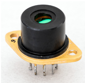
Figure 5.2.: TO3 housing with lens picture (left) and specifications (right).
