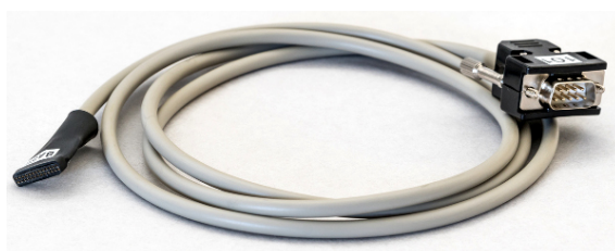
Figure 5.20.: C-LDX-LLH cable connecting the LLH housing to the LDX driver.
