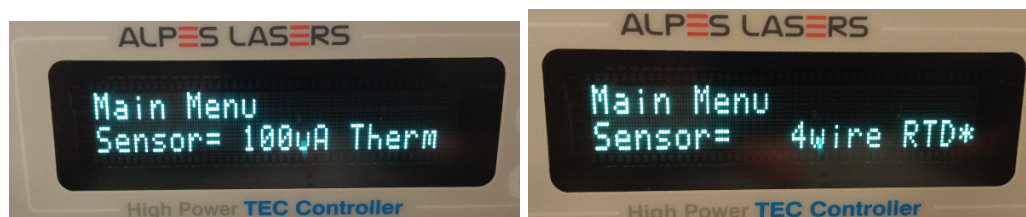
Figure 6.6.: TC-3 temperature controller GUI sensor type.
