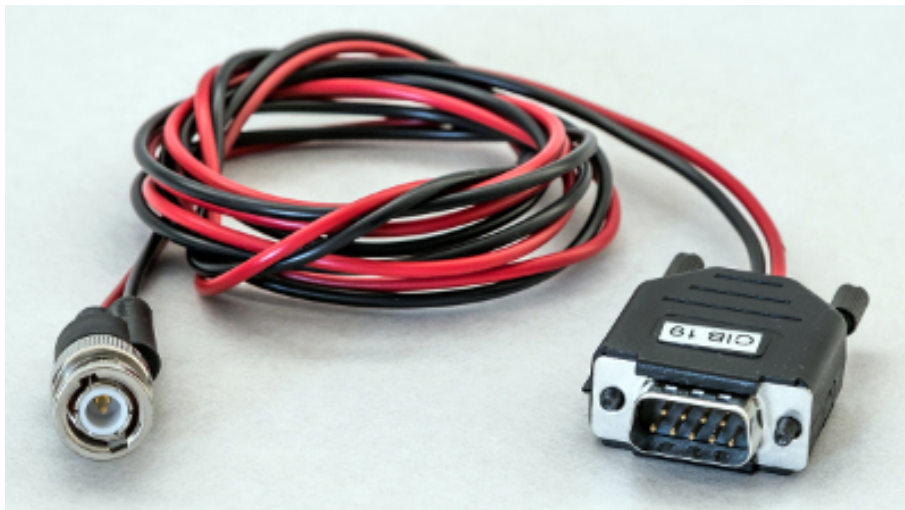
Figure 5.11.: C-LDX-HHL cable connecting the HHL housing to the LDX-3232 driver.
