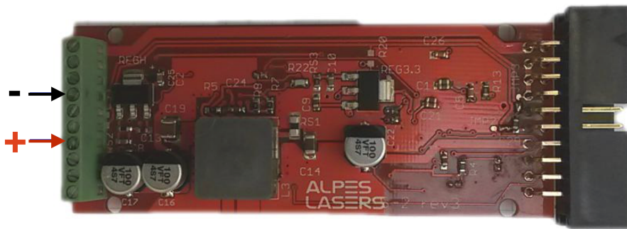
Figure 2.1: S-2 pulsed driver. Connect QCL wires to screw terminals 4 and 7 as indicated.
