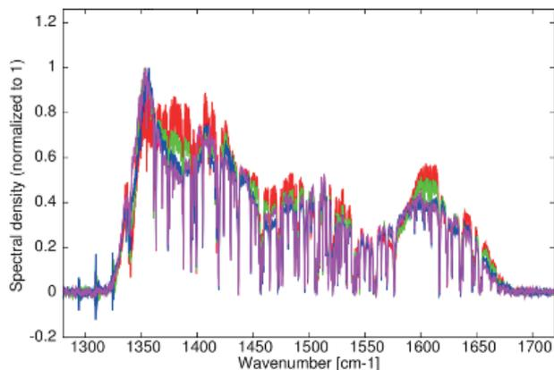
This figure shows a sample spectrum from the BG-6.2-7.4 series which shows the dense coverage that can be reached with these lasers. The different colours correspond to different temperatures of operation. The laser is pulsed in this setup. The narrow dips correspond to narrow water absorption lines in the beam path.
