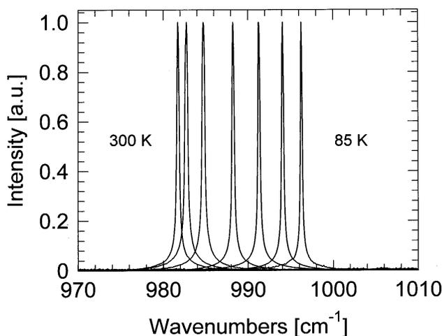
FIG. 4. Lasing spectra of a 45- $\mu\text{m}$ -wide and 1.2-mm-long DFB QC laser at different temperatures between 85 and 300 K. All spectra were measured with the maximum possible output power at each individual temperature.
