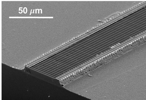
FIG. 1. (a) Schematic cross section through the laser waveguide showing the exact position of the grating with respect to the active layer and the metal top contact. (b) Scanning electron microscopy picture of a QC DFB laser. Please note that there is no metal in the central top part of the ridge waveguide.
